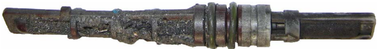
Example of contamination collected on inlet side of orifice tube requiring system flushing
